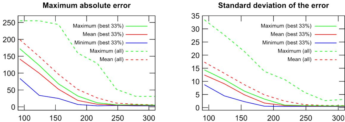
**Figure 10** Maximum absolute recovery error and standard deviation of the recovery error as a function of the number of measurements
