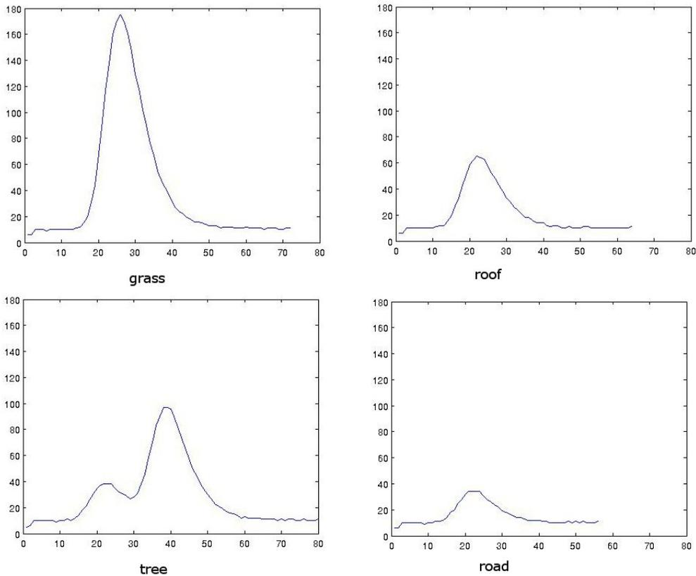
**Figure 1** Typical waveform types(x axis-time [ns] , y axis – intensity), (Courtesy of Optech Incorporated)
