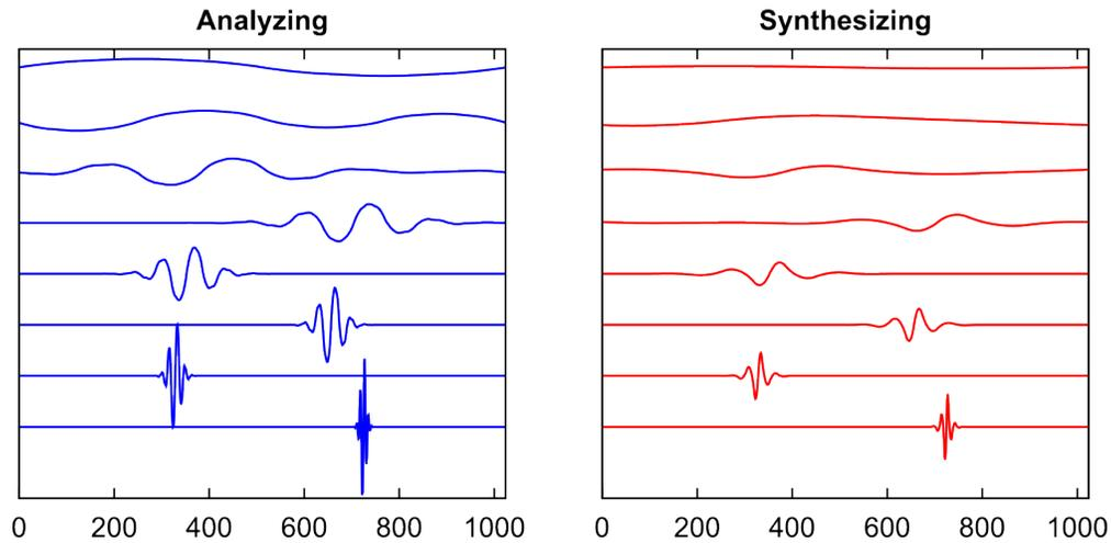
**Figure 3** Examples of CDF/3/9 analyzing and synthesizing basis functions
