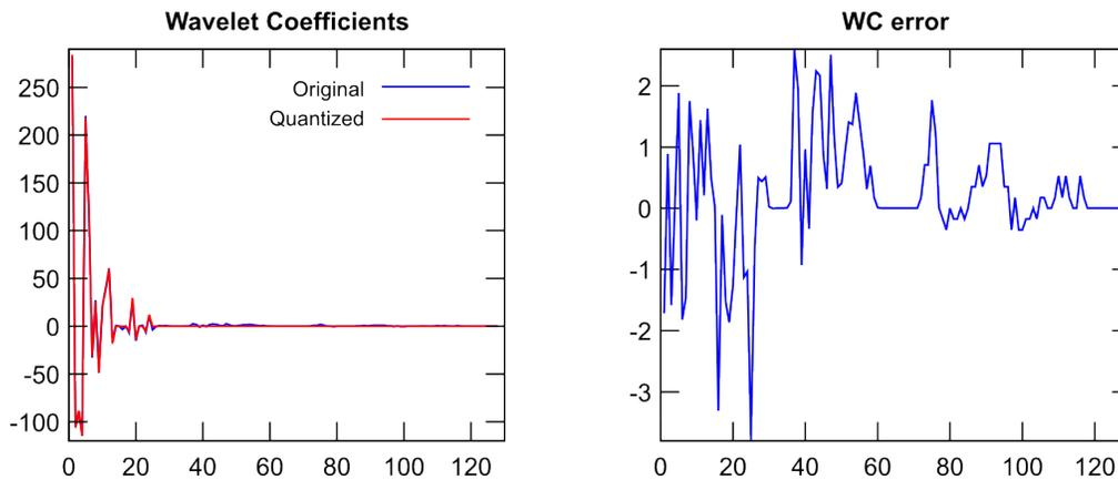
**Figure 9** Example of the effect of the quantization error on the wavelet coefficients (threshold=5.0, length of quantized wavelet coefficient vector=24)
