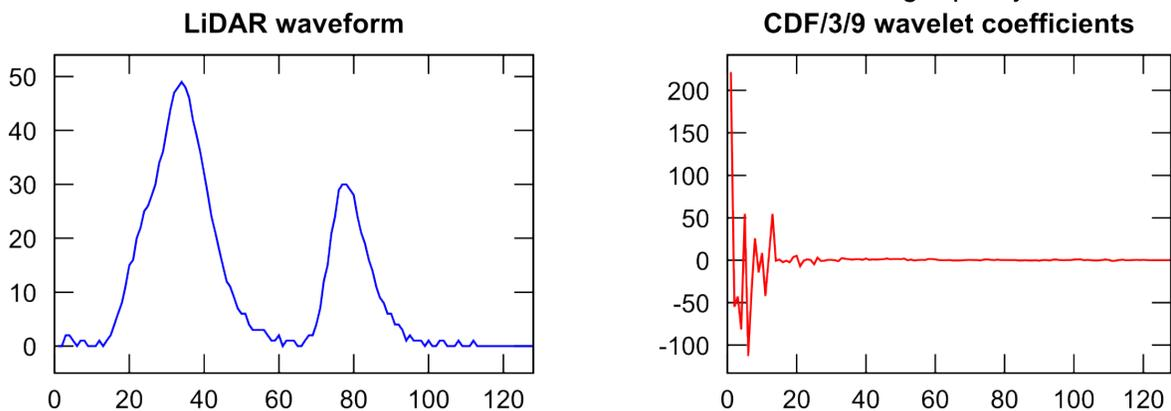
**Figure 4** Typical LiDAR waveform and its wavelet coefficients
