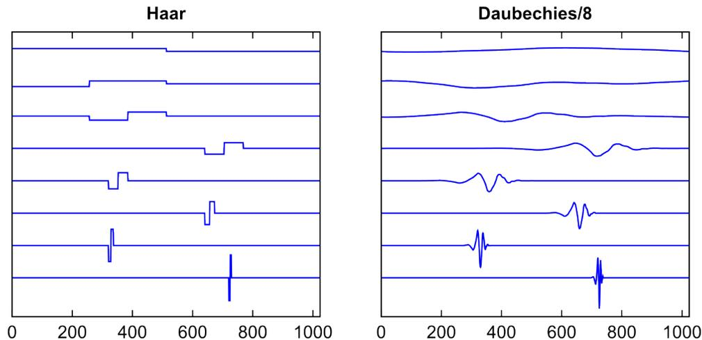
**Figure 2** Examples of Haar and Daubechies/8 wavelet basis functions
