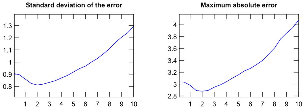
**Figure 6** Effect of wavelet coefficient (WC) quantization on the signal as a function of quantization threshold
