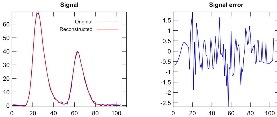
**Figure 8** Example of the effect of wavelet coefficient quantization on one signal (threshold=5.0, length of quantized wavelet coefficient vector=24, length of the original signal=104, compression rate=23.1%)
