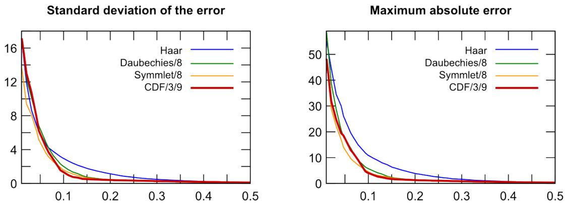
**Figure 5** Evaluation of different wavelet families with respect to compression performance
